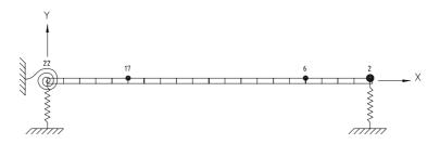
Figura 3: Analytical linear model Test Rig
