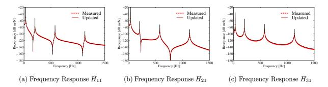
Figura 4: Frequency Responses of linear structure
