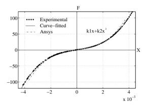
Figura 5: Relationship between loading and deformation
